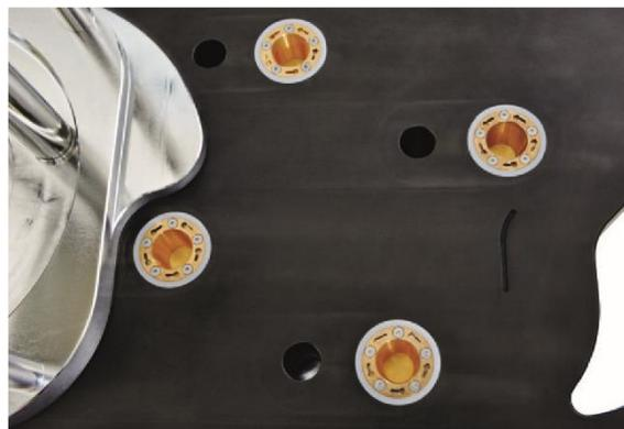
Figure 4 Baseplate showing all four microbalances in place.
