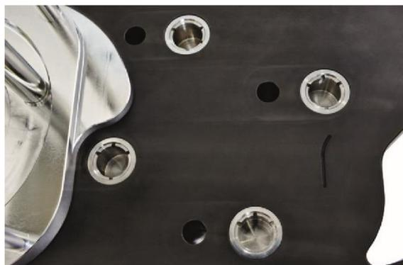
Figure 6 Base plate showing four microbalance positions replaced with four metal cups containing cell culture inserts.
