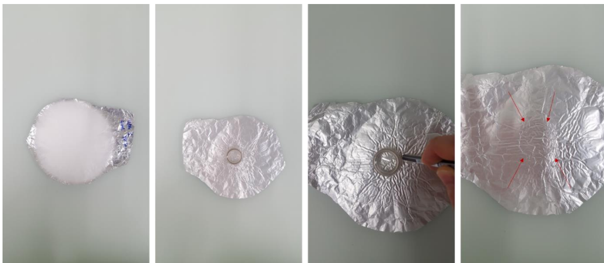
Figure 7: Picture showing the procedure to obtain a sample from a sheet of membrane material.
