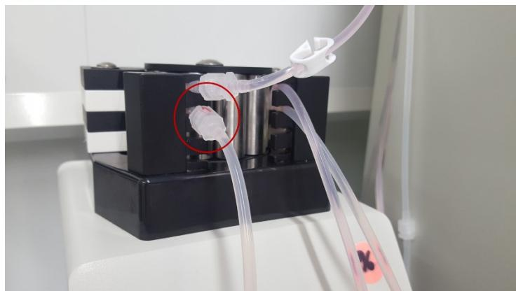
4. Connect one end of the *pump tube* to the outlet tube of the bioreactor (higher position) and the other end to the reservoir
