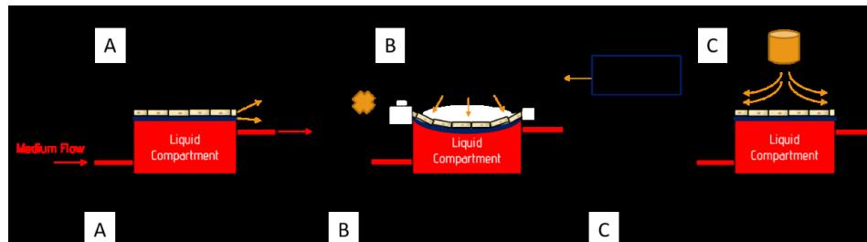
Figure 7: Key elements of the DALI system: A) ALI with media flow, B) stretching of the membrane and C) aerosol deposition on the cell layer.
