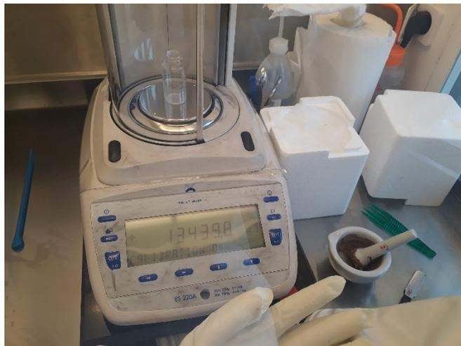
Figure 2. Mixing CeO<sub>2</sub> in chocolate spread in a glove box using mortar and pestil. The empty glass vial is weighed to ensure that all nanomaterial has been transferred to the mortar.
