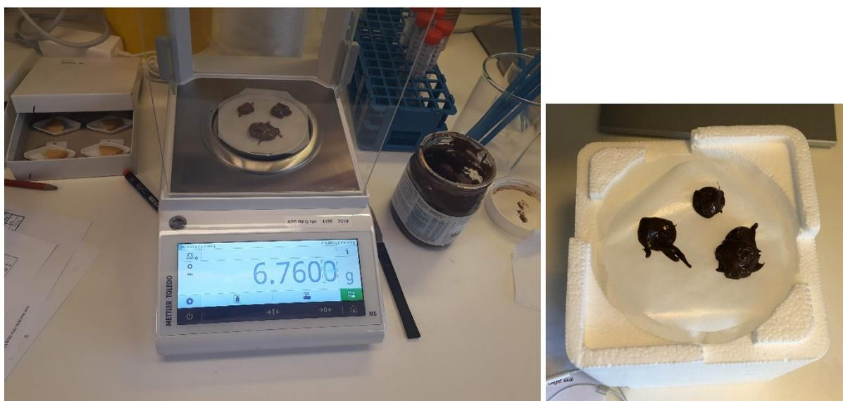
Figure 1. Portions of chocolate spread prepared on an analytical balance (left) and cooled on dry ice (right).
