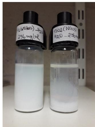
**Figure 20: Suspensions of TiO<sub>2</sub> NM-105 particles suspended in water at a concentration of 2.56 mg/mL.**
